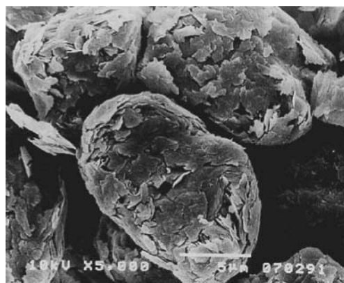
Figure 1. The SEM observation of microcrystalline talc.
